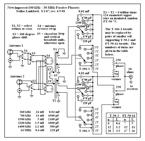
toroids specified on the schematic, two pairs of smaller self supporting toroids were used, namely T-50-2 and FT-50-61 toroids. The numbers of turns for the required inductances are given in the table with the schematic. The bandswitched version below was built to determine if this approach works well at VLF and if it is useful for
