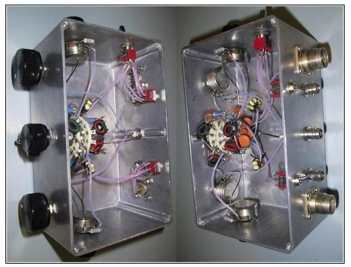
Above are interior photos of a previous version of the bandswitched 100 kHz - 30 MHz Passive Phaser. The switched inductive coupling enhancement (switch S5) was not implemented in this version. The vernier pots on the sides are 100 ohm in parallel with fixed 100 ohm resistors.
