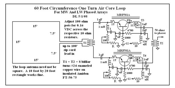
The amplified 60' circumference loop antenna above and an amplified 15' noise reducing vertical antenna are very good for null steering in the NDB band using the new improved passive phaser. They are, of course, not
